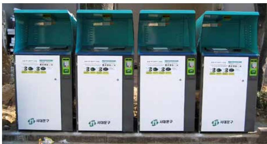
RFID-based Pay-As-You-Throw Food Waste Collection system in Seodaemun-gu, Seoul © THE FINANCIAL NEWS
